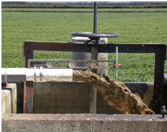
The trajectory of water being discharged from an open pipe may be used to estimate flow rate.
