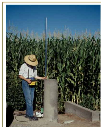
Measuring velocity in an underground pipe with an electromagnetic meter mounted on aluminum concrete finishing poles that can be snapped together to obtain the length needed.
