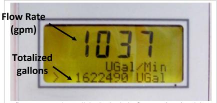
A flow meter readout will display both the flow rate (gpm) and the totalized flow (hundred or thousand gallons). The flow rate is like the speedometer, it tells how fast the water is being appliedd The totalizer is like the odometer, it tells how many gallons have passed through the meter. Ask your supplier how to access these readings if they are not already displayed.
