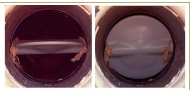
The butterfly valve on the left is shown in the open position. If debris becomes wrapped around the axis, the valve may not shut completely. The valve on the right is shown in the position needed to achieve a targeted application rate. The opening was too small to prevent frequent plugging, and the valve was subject to excessive wear from scouring and wobbling.
