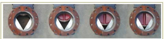
A V-notch gate valve maintains a relatively large opening for solids to pass through even when it is nearly closed, and it also makes it easier to make adjustments at lower flow rates.
