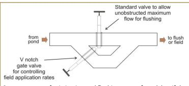
Separate pumps for irrigation and flushing are preferred, but if the same pump must be used, do not install a v-notch throttling valve on flow that will be used for flushing since it will cause an unacceptable decrease in flow rate.
