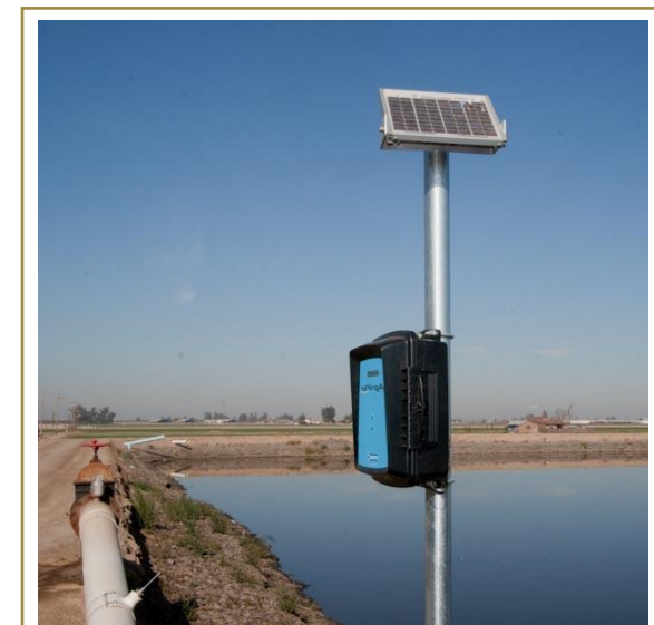
A good quality solar powered meter can eliminate most of the difficulties frequently encountered with 120V or battery operated models.
