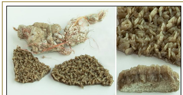
A crystalline deposit called struvite can form thick coatings on the inside of some lagoon pipelines. These will interfere with sensors that cannot be easily cleaned, and may be thick enough to change the diameter of the pipeline.
