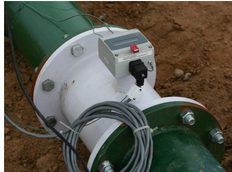
This photo shows an electromagnetic meter that replaces a section of pipe. The terms “spool type,” “tube style” and “full bore” are used interchangeably for this type of meter.
